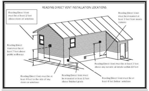
Location of the termination of venting systems should be installed in accordance with the National Solid Fuel UL Code 1482, manufacturer's recommendations and/or local codes which are applicable. See requirements below or refer to installation location, Diagram A, for typical locations.
