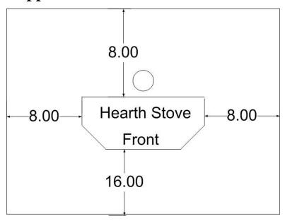
Tested 9/89 to ANSI/UL 1482, CSA B366-m1979 & ETLM 78-1 Chimney Type: Minimum 6 inch diameter approved low heat residential type all fuel. Chimney connector: 6 inch diameters 24 gauge blue or black steel.
