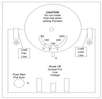
**RELAY**-receives signal from 24V thermostat to turn on or turn off gear motor.
