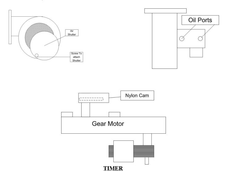
The timer is shown on the next page. The purpose of a timer is to **maintain a minimum** fire when thermostat is not calling for heat.
